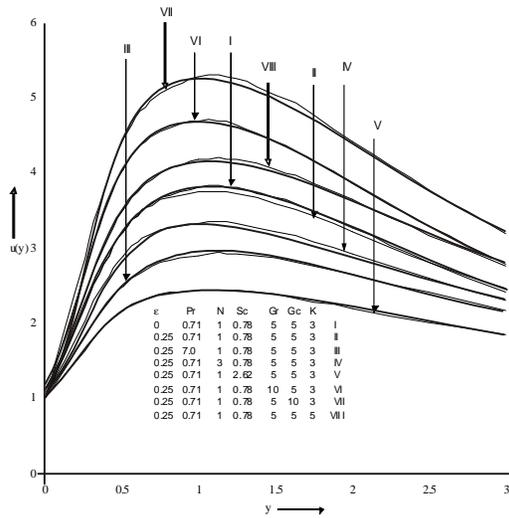
Fig. 2. Velocity distribution versus  $y$ , when  $A = 1$ ,  $Up = 1$ ,  $\delta = 0.5$ ,  $\beta = 0.5$ ,  $n = 0.5$  and  $t = 1$ .
