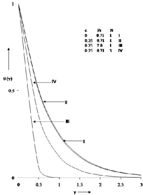
Fig. 4. Temperature distribution versus  $y$ , when  $A = 1$ ,  $\delta = 0.5$  and  $t = 1$ .
