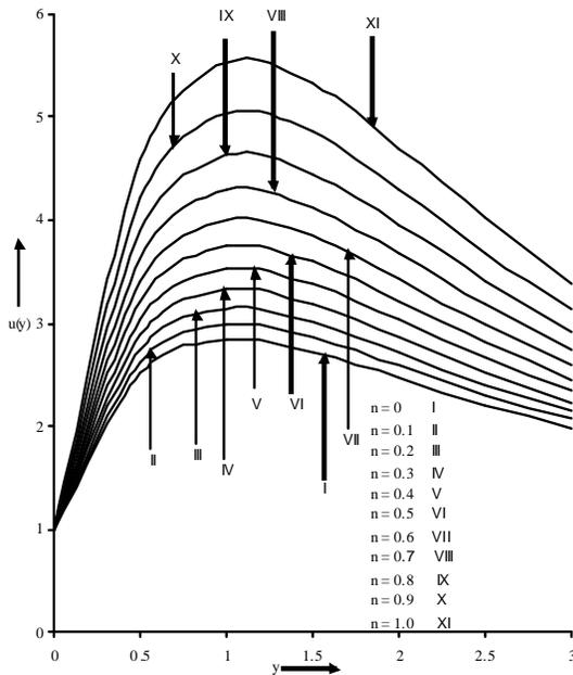
Fig. 6. Velocity distribution versus  $y$ , when  $A = 1$ ,  $Up = 1$ ,  $\delta = 0.5$ ,  $\beta = 0.5$ ,  $Pr = 0.71$ ,  $Sc = 0.78$ ,  $N = 3$ ,  $Gr = 5$ ,  $Gc = 5$  and  $K = 3$ .
